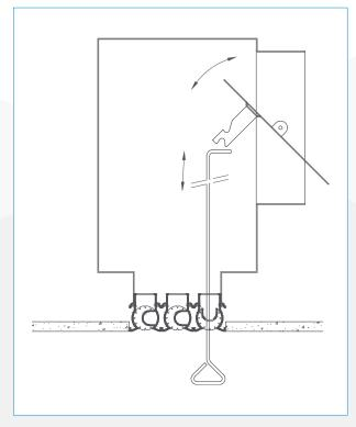
Diffuser attached directly to the plenum (fixing by Grada upon request). Volume control valve in the inlet adjustable at the front diffuser (LP310). Provided with mounting eyes, mounting straps available upon request.
