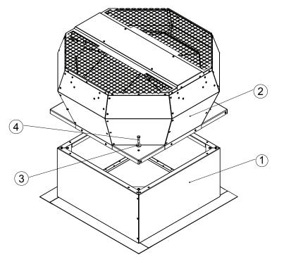
■ Fasten the roof fan (2) with screws and washers (3) and (4) on the roof socket (1)
