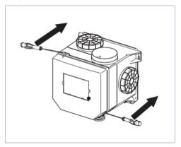
b) With the help of both potmeters the capacity in high (H) and low (L) can be adjusted.
