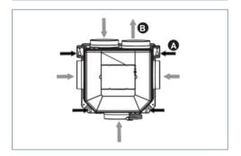
Attach the ventilation unit, preferably in a closed room, with the appropriate screws and the mounting holes to a (sloping) wall or ceiling/floor with sufficient load-bearing capacity (> 200 kg/m2). (A)
