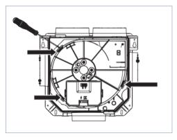
d) Remove the motor plate, complete with motor and impeller and circuit board housing.
