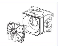
e) Clean the impeller with a soft brush. Make sure that any balancing clips remain on the impeller.
