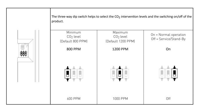
The functioning ratio of the product according to the selected configuration follows the underneath diagram:
