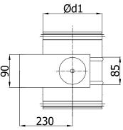
Standard: lengthwise actuator orientation
