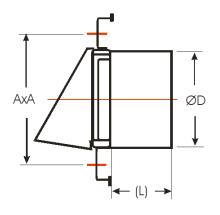
The D5 with moveable vanes are extremely solid and made of high quality 304/2B stainless steel.
